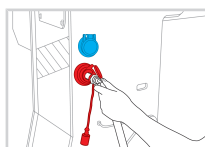
Hydraulic sockets on the boom head
