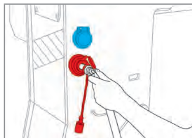
Hydraulic sockets on the boom head
