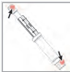
Lifting cylinder lubrication points.
