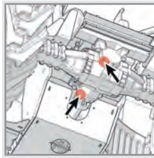
Swinging axle lubrication points.
