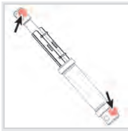
Lifting cylinder lubrication points.
