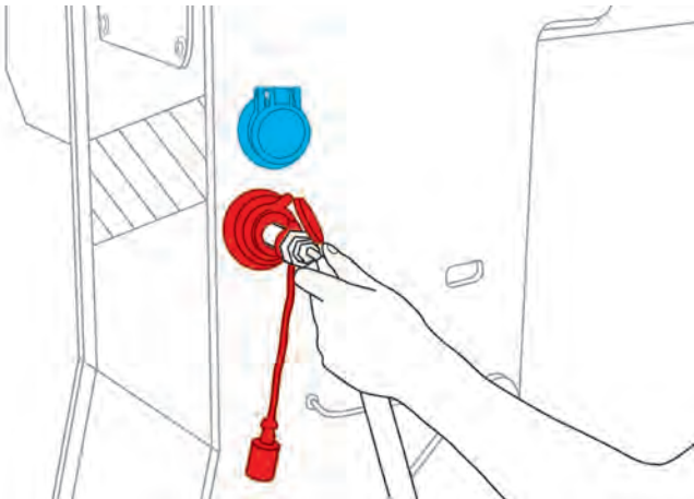
Figure: Hydraulic sockets on boom head
