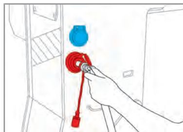
Hydraulic sockets on the boom head
