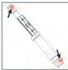
Lifting cylinder lubrication points.
