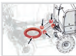
Lubrication points for drum lifting cylinders and drum rotation fifth wheel (if any).
