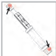
Lifting cylinder lubrication points.
