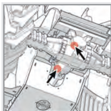
Swinging axle lubrication points.
