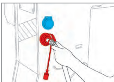
Hydraulic sockets on the boom head
