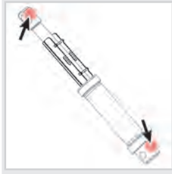
Lifting cylinder lubrication points.
