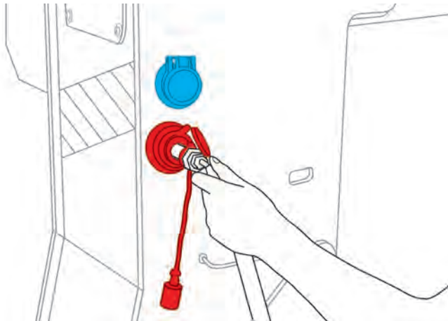
Figure: Hydraulic sockets on boom head
