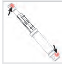
Lifting cylinder lubrication points.
