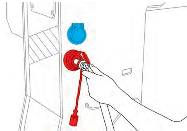
Figure: Hydraulic sockets on boom head
