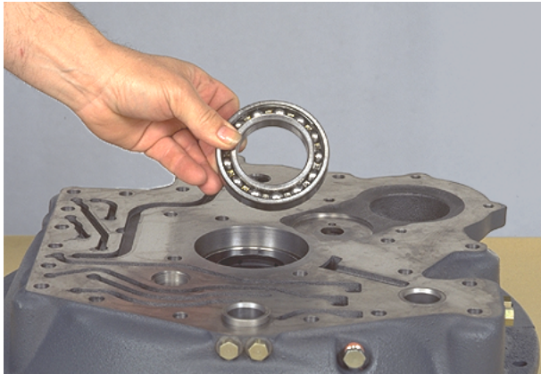
Figure 353 Remove torque converter bearing.
