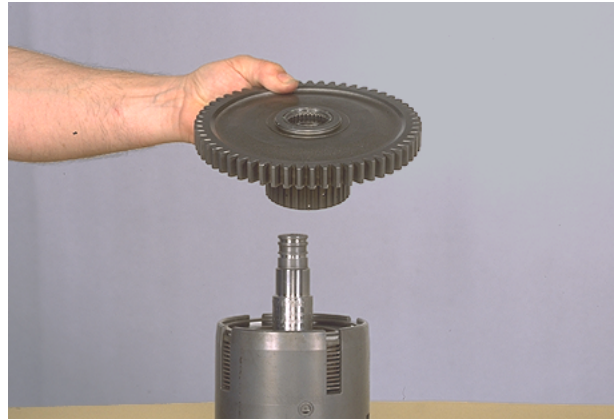
Figure 62 Remove clutch gear and disc hub.
