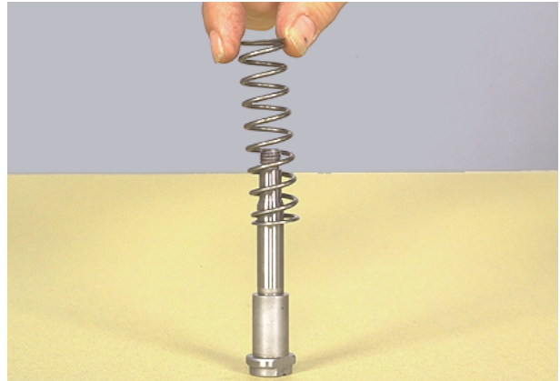
Figure 37 Remove inching return spring.
