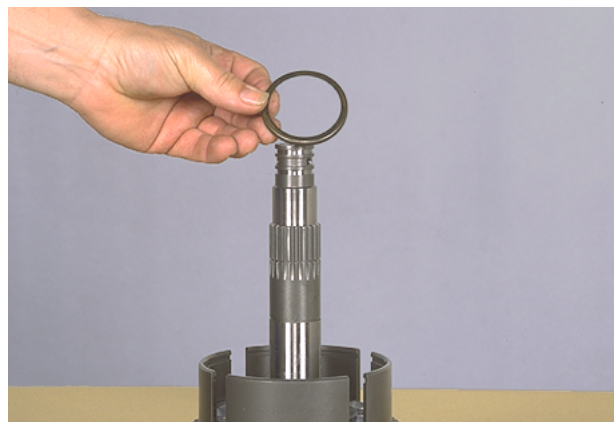
Figure 153 Remove clutch piston wear plate.
