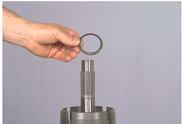
Figure 90 Remove clutch piston wear plate.
