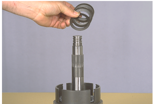
Figure 152 Remove disc springs. NOTE: see page 10-85.
