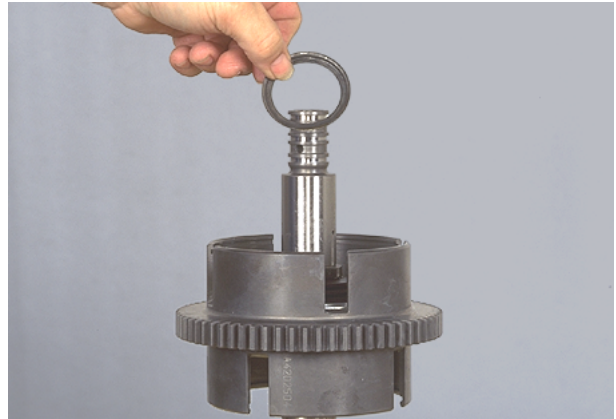
Figure 235 Remove retainer ring retainer.
