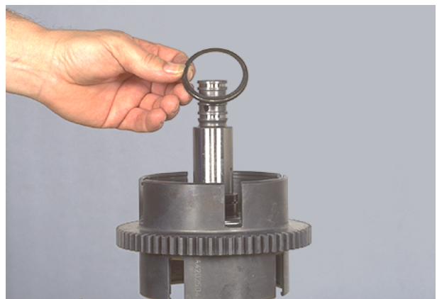
Figure 237 Remove clutch piston wear plate.
