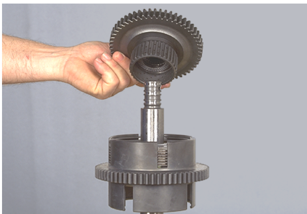
Figure 228 Remove clutch gear and disc hub.
