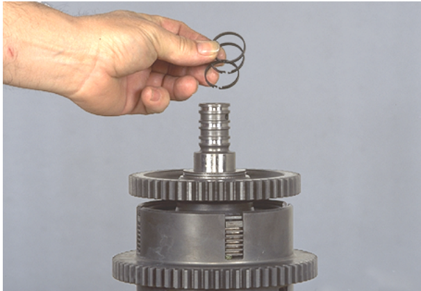
Figure 226 Remove clutch shaft oil sealing rings.
