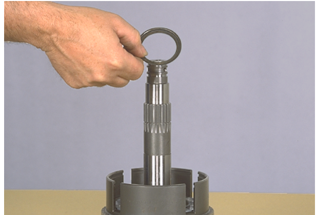
Figure 151 Remove retainer ring retainer.
