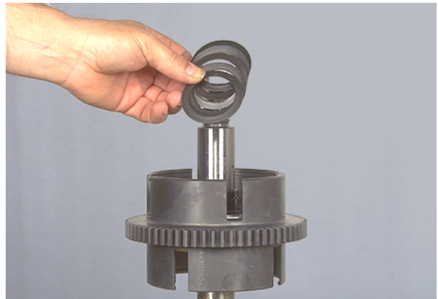
Figure 236 Remove disc springs. NOTE: see page 10-85.
