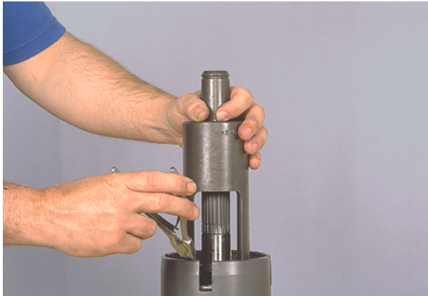
Figure 86 Compress disc springs and remove retainer ring.
