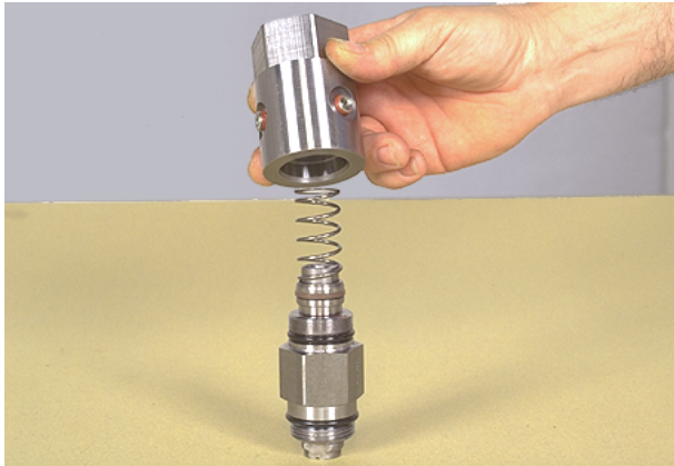
Figure 28 Remove hydraulic inching cover.
