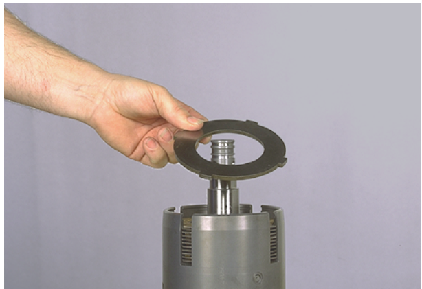
Figure 102 Install clutch disc end plate.
