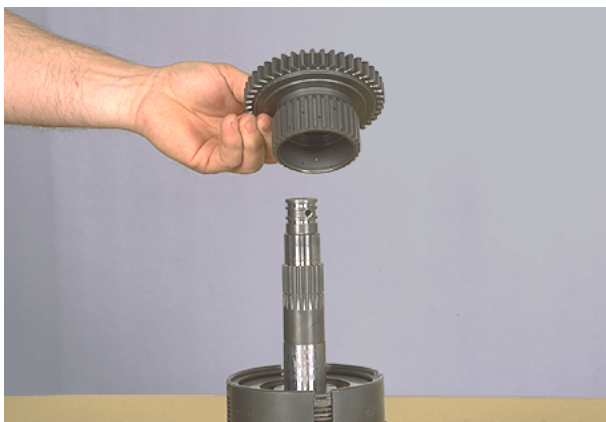
Figure 144 Remove clutch gear and disc hub.
