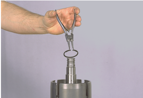
Figure 98 Start ring on shaft with snap ring pliers.
