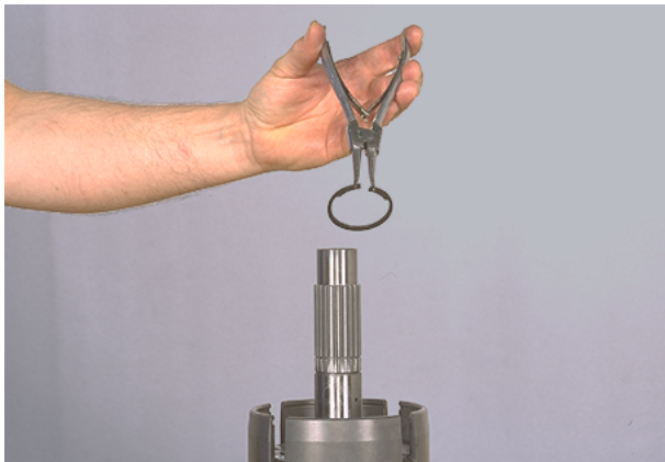
Figure 87 Remove retainer ring.
