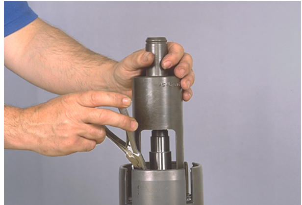
Figure 68 Compress disc springs and remove retainer ring.
