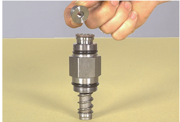
Figure 31 Inching upper piston removed.
