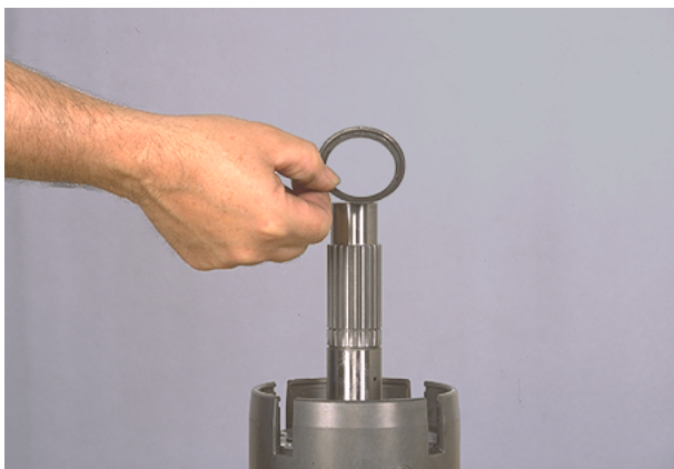
Figure 88 Remove retainer ring retainer.
