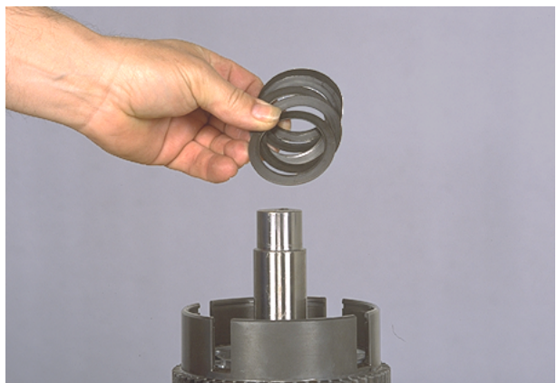
Figure 166 Remove disc springs. NOTE: See page 10-85.
