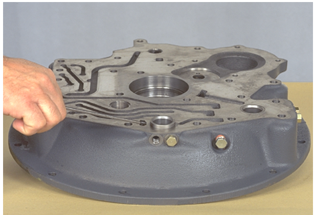
Figure 357 Remove oil distributor sleeve set screw.
