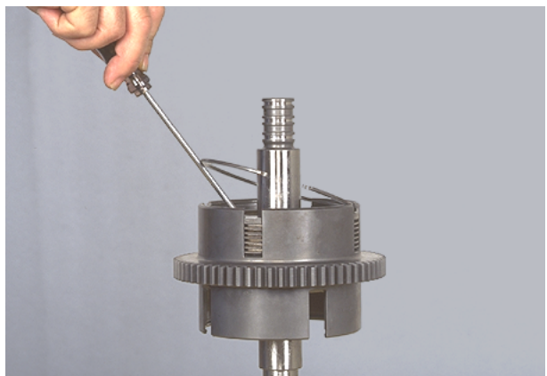
Figure 231 Remove end plate retainer ring.
