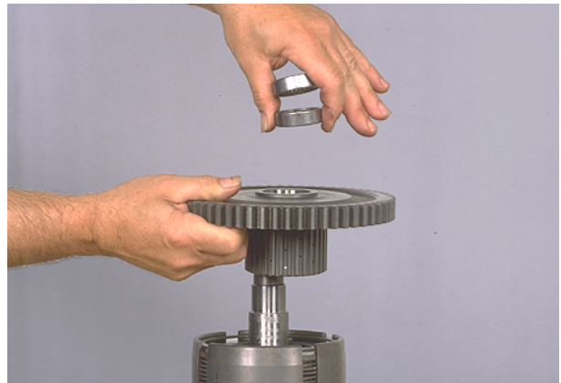
Figure 63 Clutch gear and pilot bearings removed.
