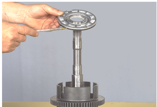
Figure 225 Remove clutch piston.
