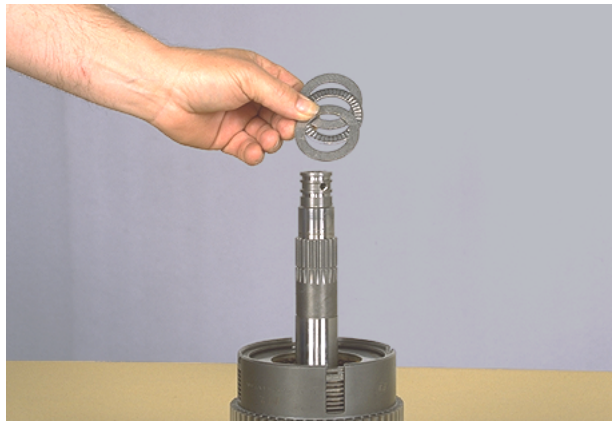
Figure 146 Remove outer thrust washer, thrust bearing and inner thrust washer.
