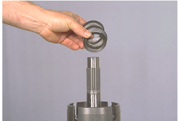
Figure 89 Remove disc springs. NOTE: see page 10-85.
