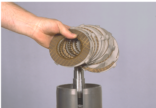
Figure 67 Remove inner and outer clutch discs.
