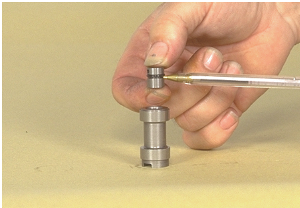
Figure 17 Remove regulator spool sleeve assembly. Remove "O"-ring.
