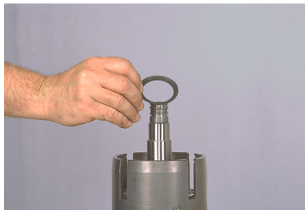
Figure 70 Remove retainer ring retainer.
