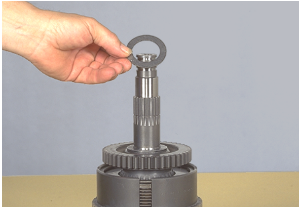
Figure 187 Position thrust washer on shaft.
