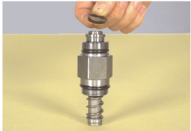
Figure 32 Remove hydraulic piston seal.
