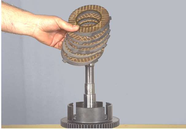
Figure 220 Remove clutch discs.
