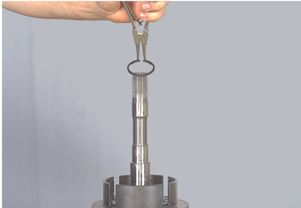
Figure 221 Compress disc springs and remove retainer ring.
