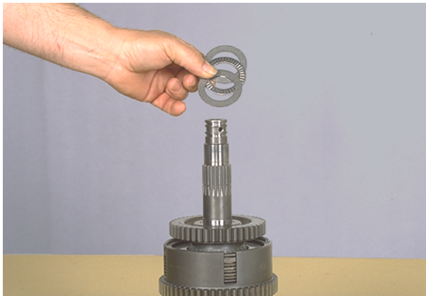
Figure 143 Remove outer washer, thrust bearing and inner thrust washer.
