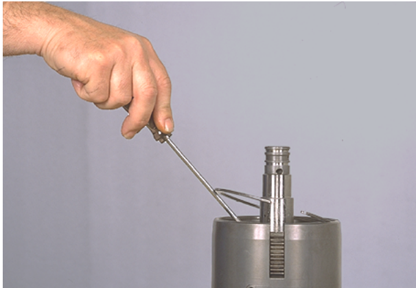
Figure 65 Remove clutch disc end plate retainer ring.
