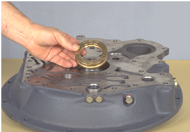
Figure 354 Remove oil distributor.
