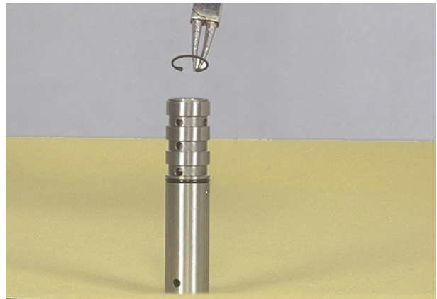
Figure 14 Remove regulator spool assembly retainer ring.
