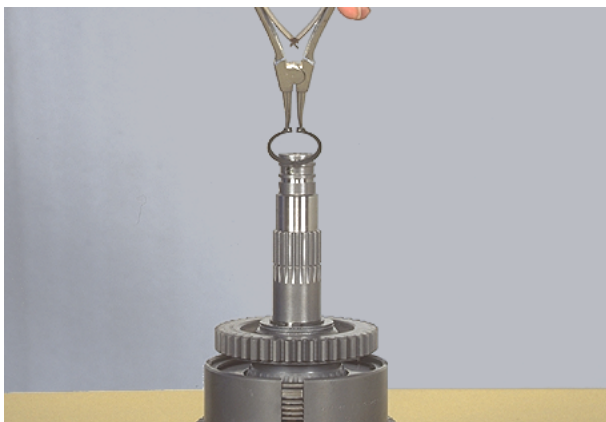
Figure 189 Install clutch shaft gear locating ring.
