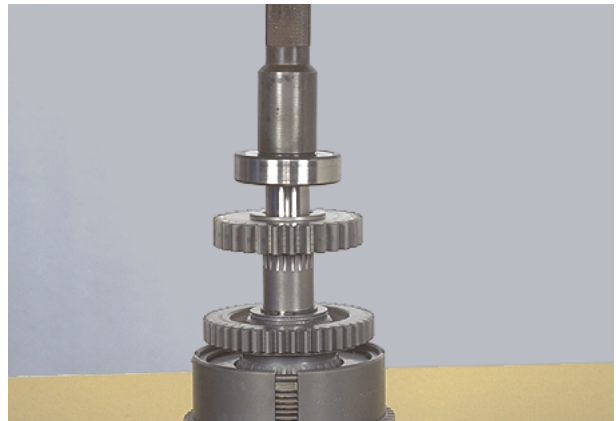
Figure 191 Install clutch shaft front bearing. Note bearing has a shield in it. This shield must be up.
