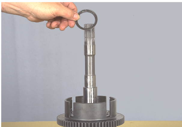
Figure 222 Remove retainer ring retainer.
