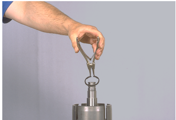
Figure 69 Remove retainer ring.
