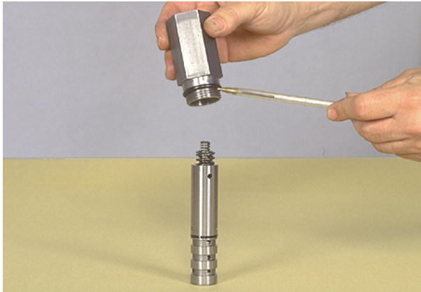
Figure 10 Remove modulator valve body "O"-ring.
