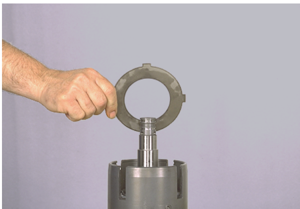
Figure 100 Install first steel outer clutch disc.
