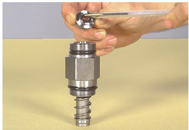
Figure 33 Remove inching lower piston and "O"-ring.
