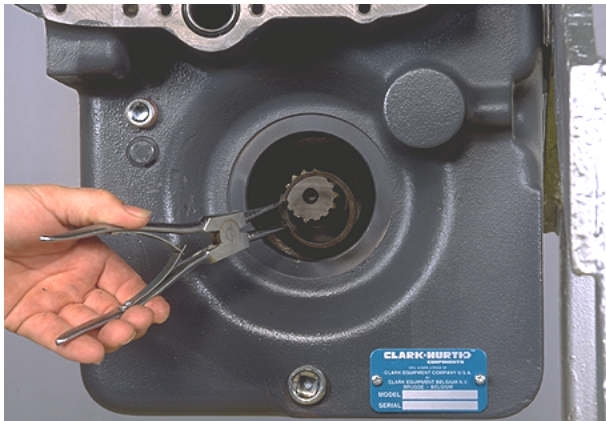
Figure 38 Remove output gear to shaft retainer ring.
