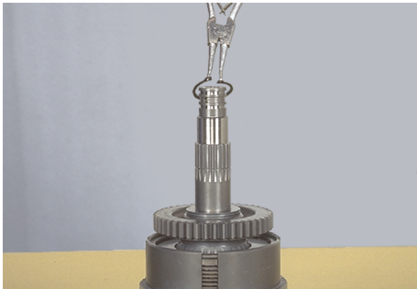
Figure 188 Install thrust washer retainer ring NOTE: 3-speed clutch drum not as shown.
