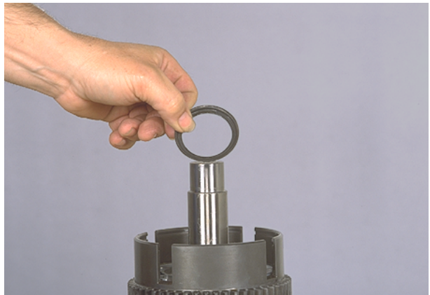
Figure 165 Remove retainer ring retainer.
