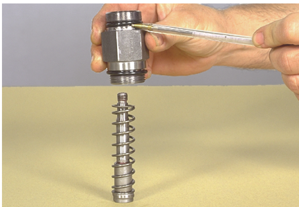
Figure 36 Remove hydraulic inching body and "O"-rings.
