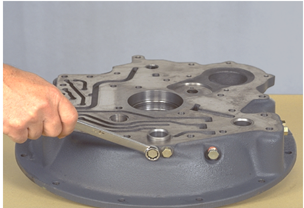
Figure 356 Remove converter housing plug (high and 3rd clutch shaft).
