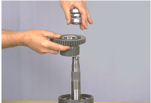
Figure 145 Remove bearings and spacer from clutch gear.
