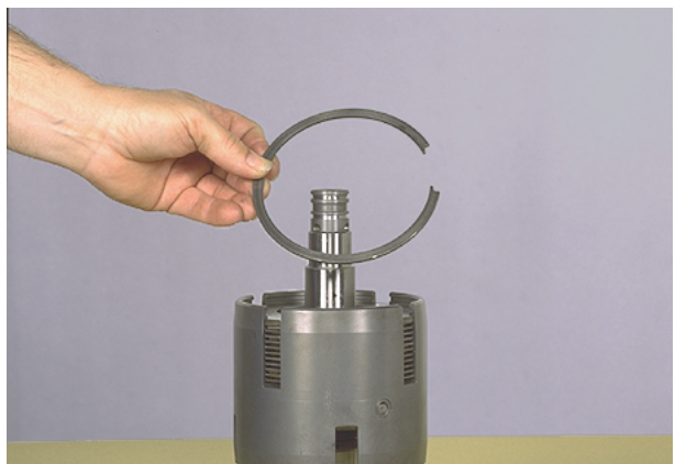
Figure 103 Install end plate retainer ring.
