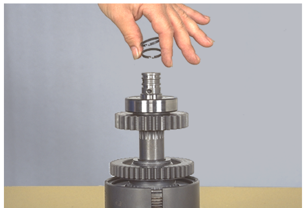
Figure 192 Install clutch shaft oil sealing rings. Grease rings to facilitate reassembly into front housing.
