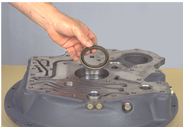
Figure 355 Remove converter oil seal.
