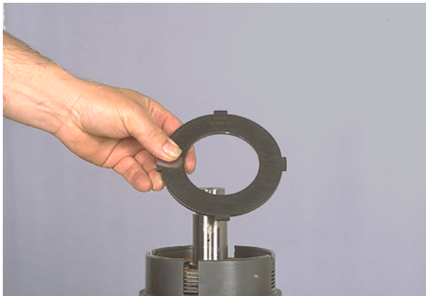
Figure 162 Remove end plate.
