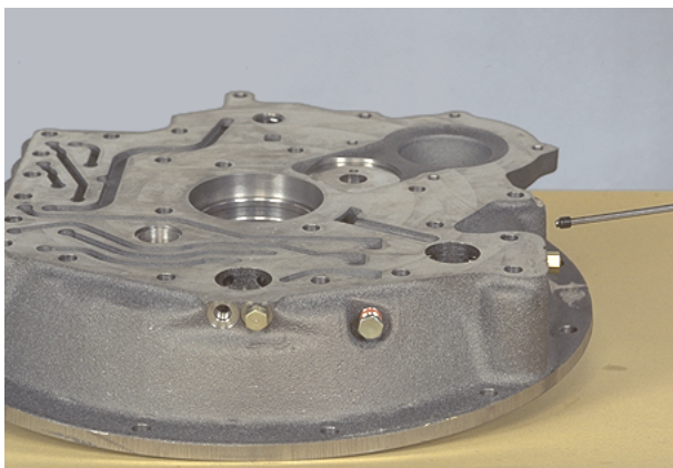
Figure 361 Remove oil distributor sleeve set screw.
