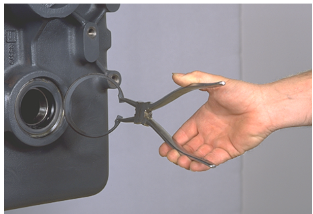
Figure 42 Remove flange oil seal sleeve retainer ring.
