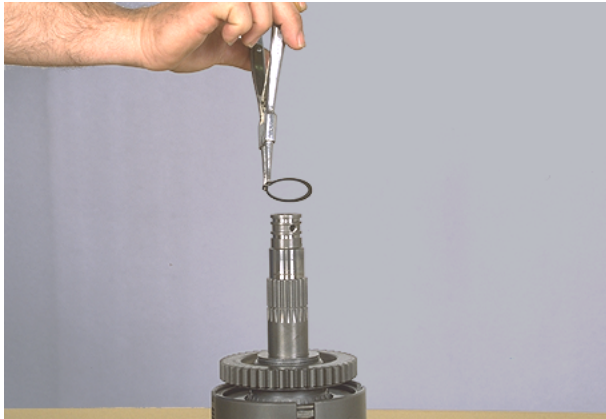
Figure 142 Remove outer thrust washer retainer ring.
