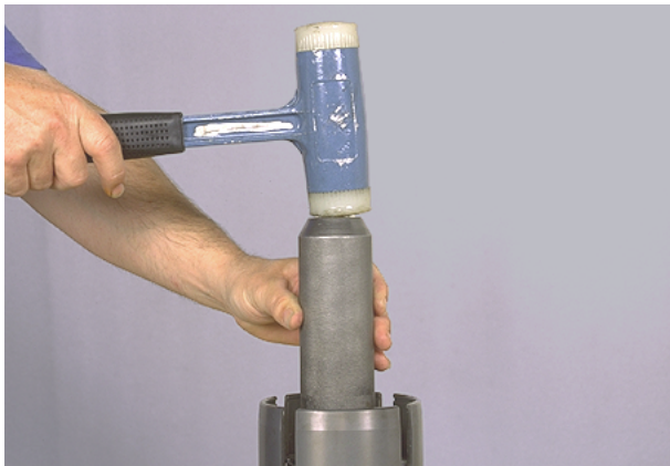
Figure 99 Use a sleeve with the proper inner diameter to fit over shaft and against retainer ring. A sharp blow with a soft hammer will compress springs and seat retainer ring. Be sure ring is in full position in groove.
