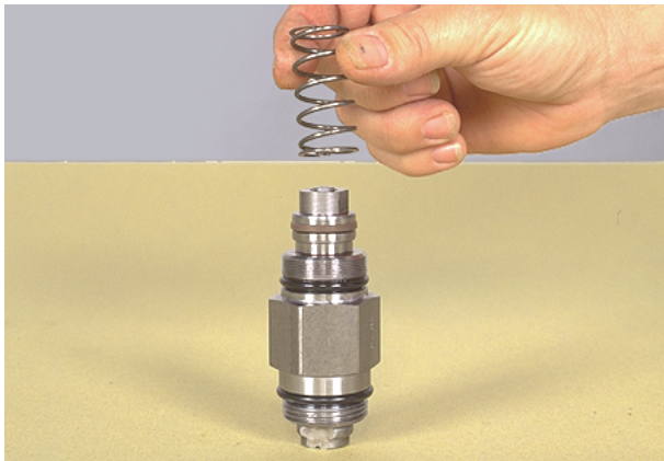
Figure 29 Remove inching return spring.
