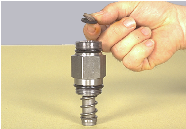
Figure 35 Remove hydraulic inching body seal.
