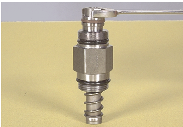
Figure 30 Remove hydraulic inching upper piston.
